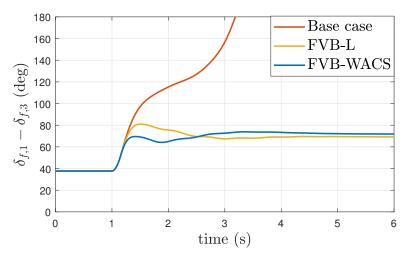
Figure 9: Fault I cleared after 150 ms. Angle difference of the VSCs.
