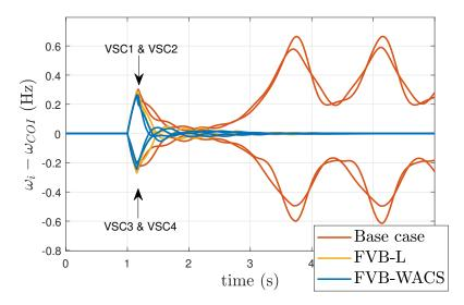
Figure 10: Fault I cleared after 150 ms. Frequency deviations of the VSCs with respect to the frequency of the COI.
