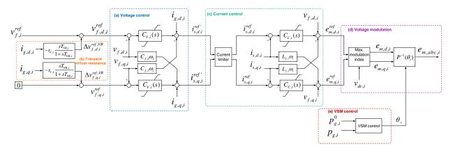
Figure 2: General scheme of the control system of a grid-forming VSC.
