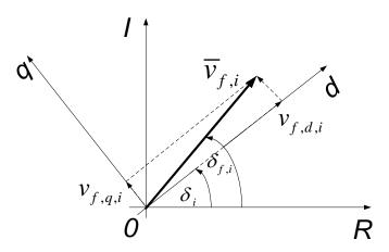
Figure 3: Grid-forming VSC: d - q axes.
