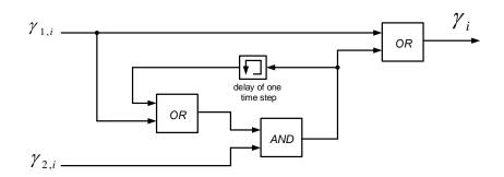
Figure 6: Strategy FVB-L. Logic circuit for fault detection.
