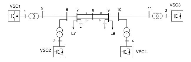
Figure 8: Kundur's two-area test system with 100 % of GF-VSC-based generation.
