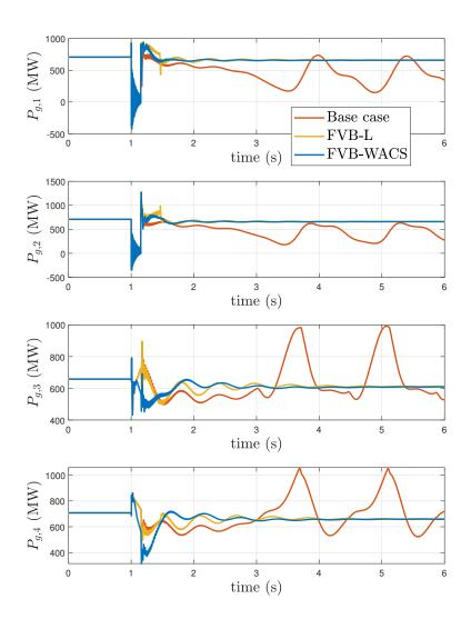
Figure 12: Fault I cleared after 150 ms. Active-power injections of the VSCs.
