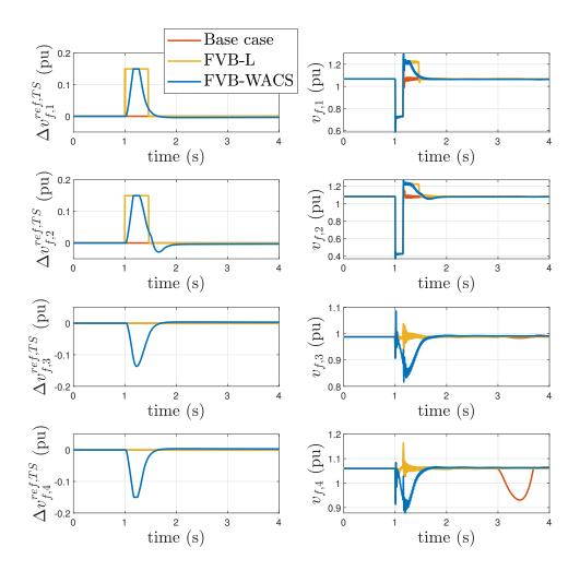
Figure 11: Fault I cleared after 150 ms. (left) Supplementary voltage set points of the VSCs and (right) voltages of the VSCs.
