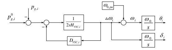
Figure 4: Supplementary controller of a virtual synchronous machine (VSM) implemented in a GF-VSC.
